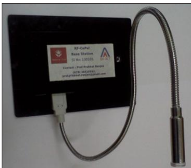
Figure 2: Base Station with one of the Flexi-Tube LED Shown. Up to Four Such LEDs can be Connected
