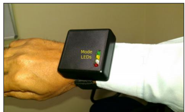
Figure 3: Final Version of the Hand Device with Four LED Indicators
