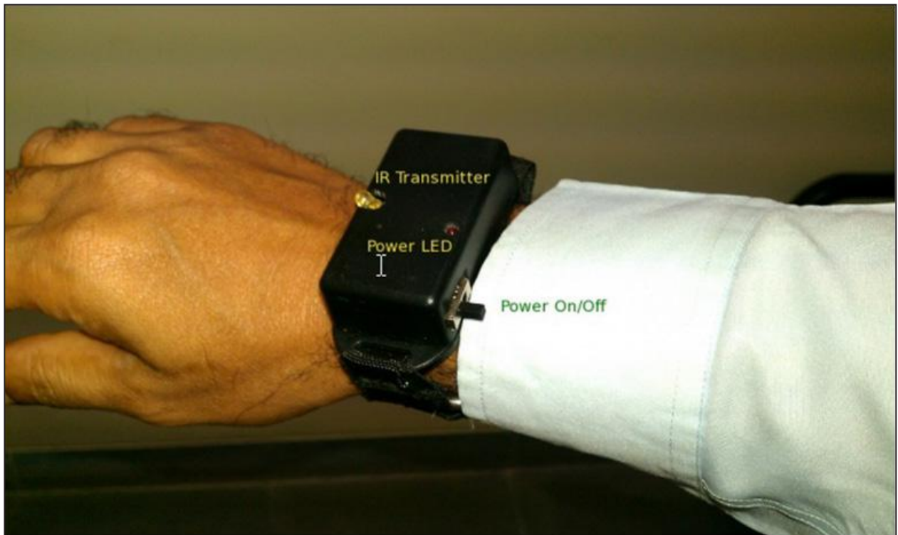
Figure 1: Mini-CePal : Single Piece Device - Needs to be Pointed Towards the Equipment
